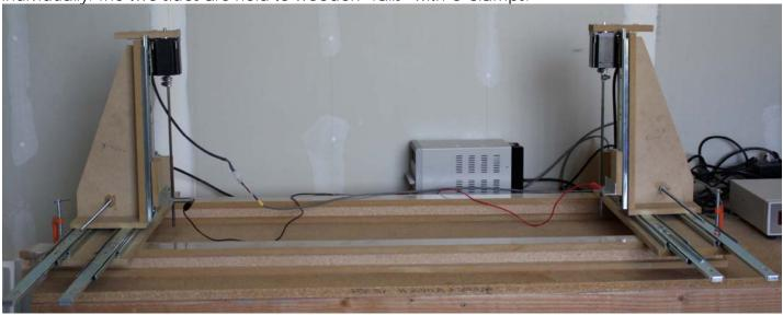
This allows me to adjust the machine to cut any size wings I want. Each side has its own horizontal and vertical axis to move on. I used full extension drawer slides to guide the motion of each axis. Each axis is moved by a length of ¼ inch 20 TPI threaded rod attached to a stepper motor, and a nut. A length of 30 gauge nichrome wire is suspended between the two sides of the machine. A spring on one side keeps the wire in tension.
